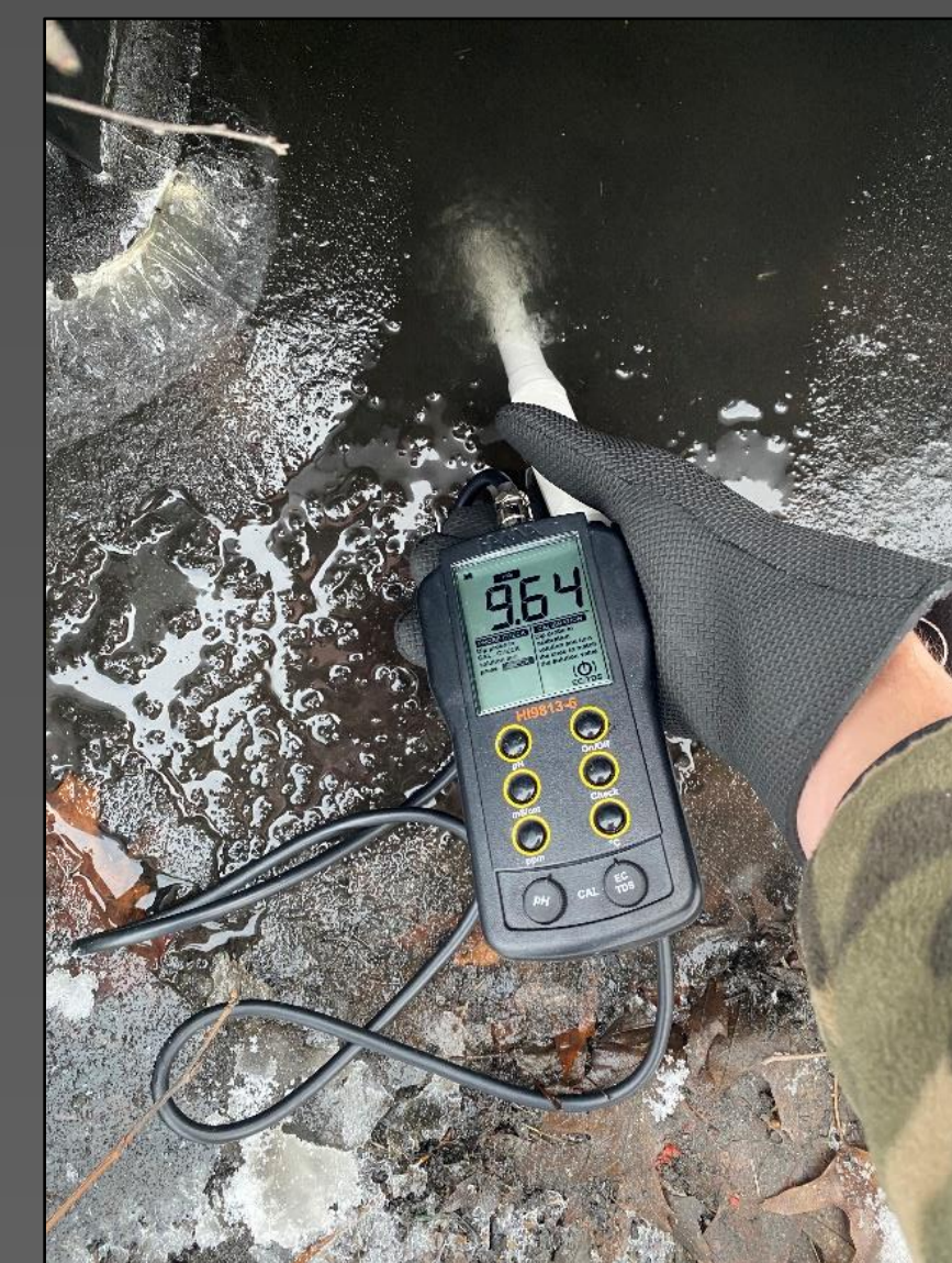
Figure 5. Conductivity being measured in mS/cm at the pond inflow with the handheld probe.
