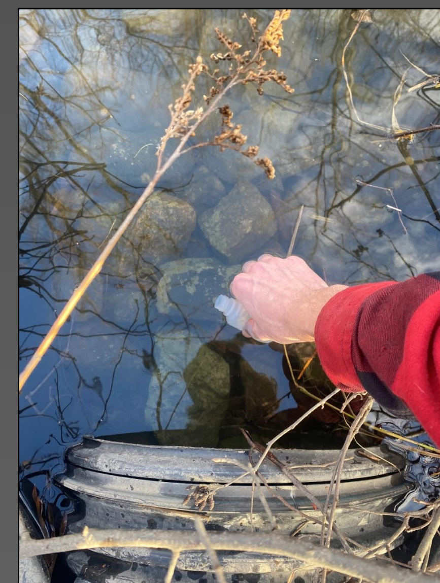
Figure 6. A water sample being collected at the outflow of the pond before it reaches the Merrimack River.
