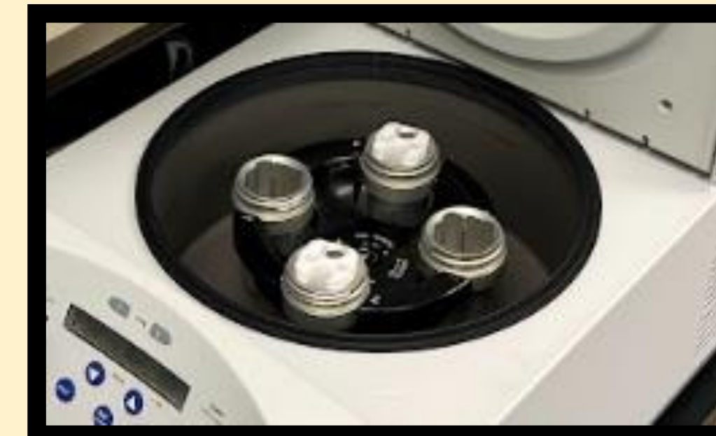
Figure 7: Centrifuge to separate trypsin from cells
