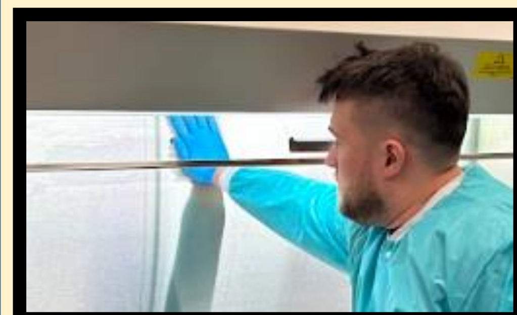
Figure 2: Start with the top and back surfaces
