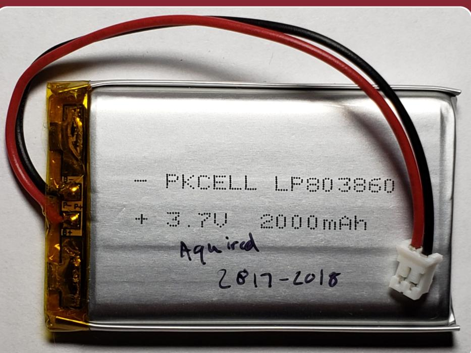
The battery shown is called a lithium polymer battery that can be recharged within a few short hours. It can also be replaced should the user want a larger capacity.
