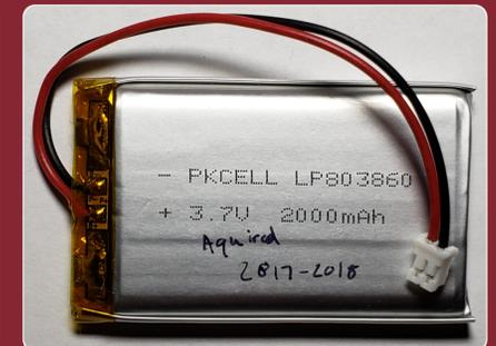
The battery shown is called a lithium polymer battery that can be recharged within a few short hours. It can also be replaced should the user want a larger capacity.
